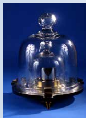
The copy of the standard kilogram in the United States is kilogram 20, produced in 1884.
