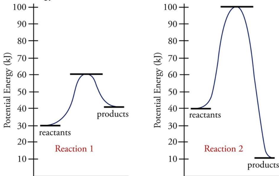
*The approximate activation energy for reaction 1 is 30 kJ and for reaction 2 is 60 kJ. Reaction 1 is endothermic, and reaction 2 is exothermic.*
