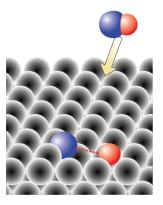
Step 1 - The reactant molecules are adsorbed, and the bonds are weakened.
