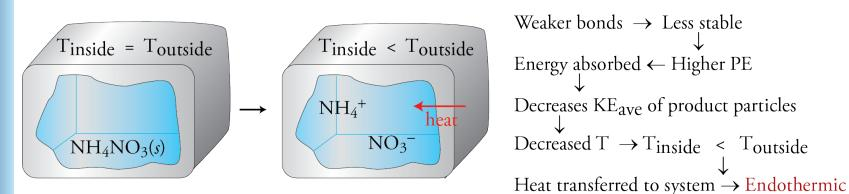
Weaker bonds  $\rightarrow$  Less stable Energy absorbed ← Higher PE Decreases KE<sub>ave</sub> of product particles Decreased  $T \rightarrow T_{inside} < T_{outside}$
